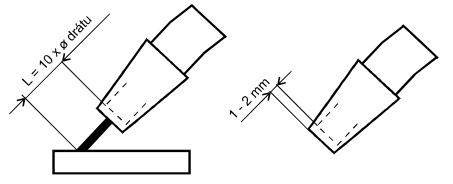
Fig. 11 – Distance from nozzle to material
