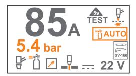
2. Also, the manual adjustment of the cutting gas pressure can be adjusted from the control panel.
