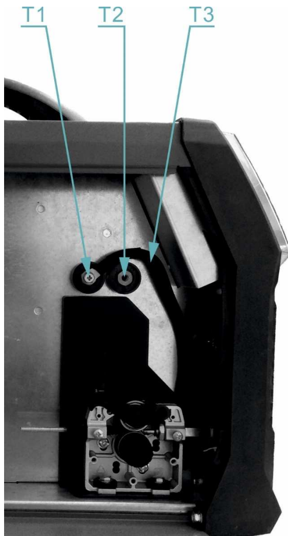
Figure 7 – Terminals for changing the polarity of the MIG/MAG torch
