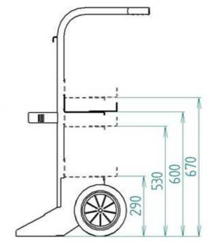
To change the shelf height, loosen the 4 screws that hold the shelf. Place the shelf in the desired position screw the screws again.
