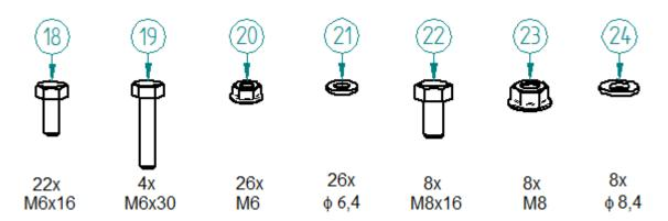
There may be more fastening components than it would be necessary. There may be different types of fasteners than stated in this manual.
