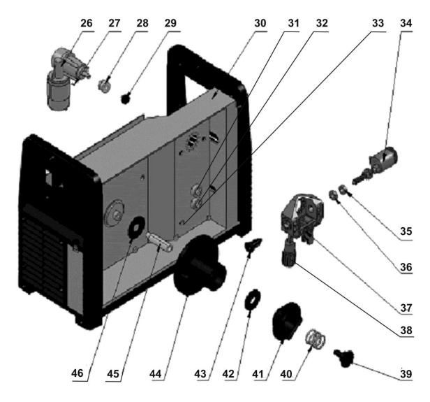
Fig. 4 – Feeding mechanism and spool holder
