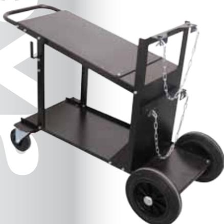
The welder's cart P80 is designed to carry every type of portable inverters (including cooling unit). The cart for welding inverter is designed to hold inverter welders, accessories and gas cylinders and handling them for short distances. The cart can hold just one gas cylinder with a maximum diameter of 20 cm and a maximum height of 120 cm. The total weight to load onto the cart is 80 kg.
