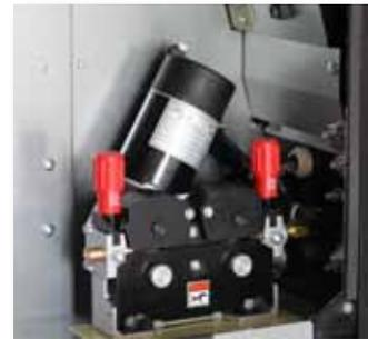
**Inner feeding lighting** - a strong LED effectively illuminates the interior and makes it easy to replace the wire in poor lighting conditions.
