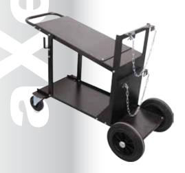
The welder's cart P80 is designed to carry every type of portable inverters (including cooling unit). The cart for welding inverter is designed to hold inverter welders, accessories and gas cylinders and handling them for short distances. The cart can hold just one gas cylinder with a maximum diameter of 20 cm and a maximum height of 120 cm. The total weight to load onto the cart is 80 kg.
